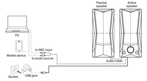
Fig. 2. Connection diagram
