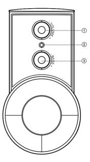
Fig. 1. Subwoofer control panel
