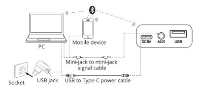
Fig. 2. Connection diagram
